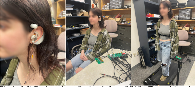
Fig. 4. (left) Earphone data collection platform. (Middle) The participant is at rest. (Right) The participant is walking. Groundtruth ECG chest strap collects data simultaneously with the earbuds.
