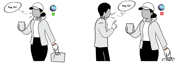
Figure 1: A few representative examples of EarVoice. (left): EarVoice allows mobile users to activate their voice assistant without hand intervention. (right): EarVoice can automatically detect the primary speaker, avoiding false alarms.
